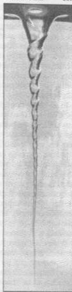
Vortex photographed underwater reveals the spiraling surface between the water and the air which is being sucked in. (Photo by Theodor Schwenk, Sensitive Chaos )
